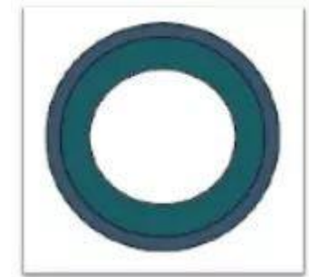
Bottoming Effect (Sulfur Dye + Indigo)
