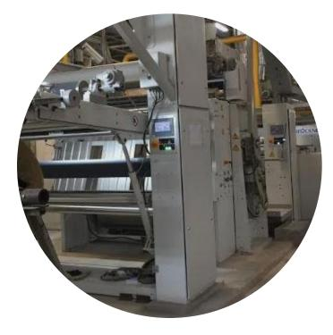
Typical operations before colouring are washing and thermofixing (heat-setting)
