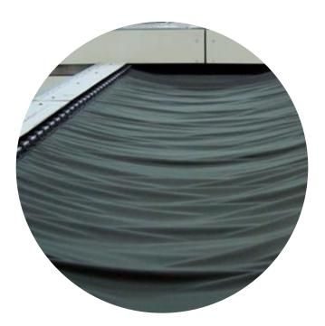
This machine is used for full drying of the fabric. The fabric is conveyed through the machine in open width. A hot current of air is blown across the fabric thereby producing evaporation of the water.
