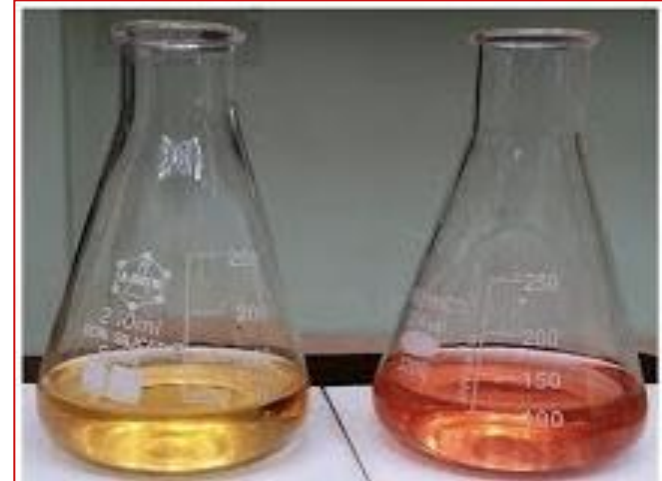
Methyl orange alkalinity: After addition of methyl orange indicator and at end point.
