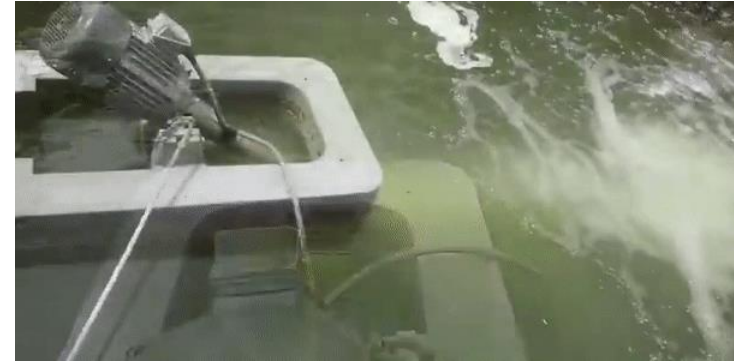
Jet aerator mounted on floats (Blowtac)
