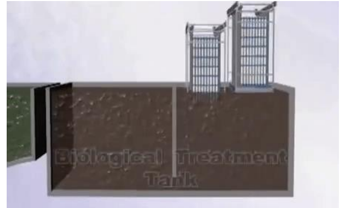
Submerged MBR with placement of membranes; photo: Courtesy Koch
