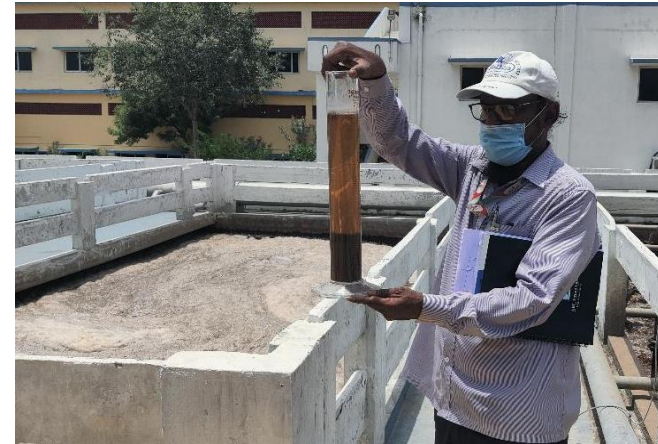
Observing the settling in aeration tank - one of the most important checking by operator
