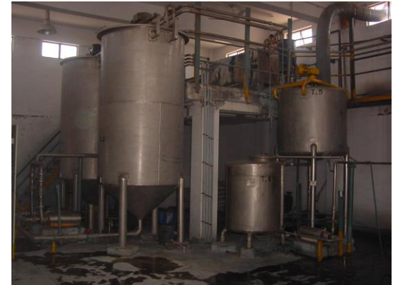
Chrome recovery system in a tannery, Source: UNIDO Leather Panel
