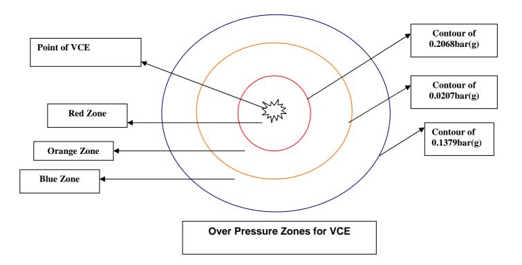
Like BLEVE, the very first zone is the "Red Zone". In this the pressure level varies from maximum (at ignition point) to the 0.2068 bar (g). Thus it stretches from the point of ignition to contour representing the pressure level of 0.2068 bar (g). The pressure level of this zone is sufficient to cause collapse of buildings; steel frame buildings can be distorted and can be pulled away from foundations.
