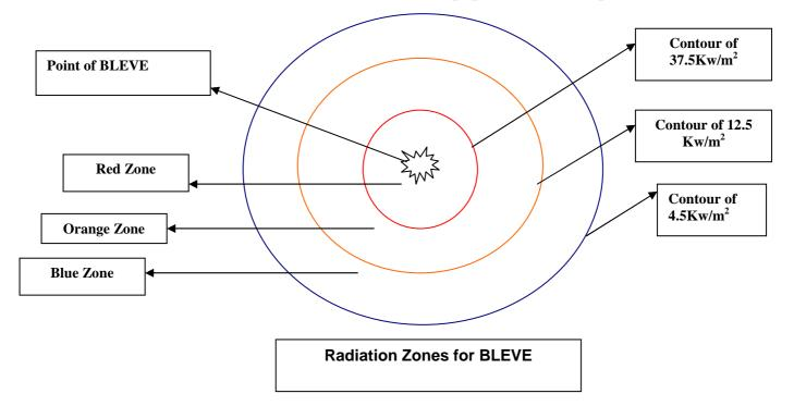
The third zone that is considered to be safer than the red and orange zone is the "Blue Zone". It extends from the contour with radiation level of  $12.5 \text{Kw/m}^2$  to the contour with radiation level of  $4.5 \text{Kw/m}^2$ . In this zone the human body may suffer the 2<sup>nd</sup> degree burn injuries if unable to reach in cover with in 20 seconds. The buildings and the industries may suffer the local fires due to liquid rainout.
