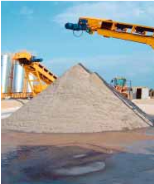
More than 20,000 tons of pretreated sludge (limed and pressed) were fed into the kiln lines of Holcim France-Benelux.
