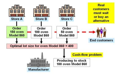
Figure 14: Negative effects of waiting for orders to produce large batches
