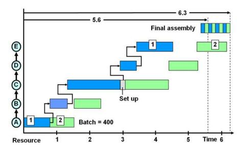
Figure 9: Production with "optimal" batch size
