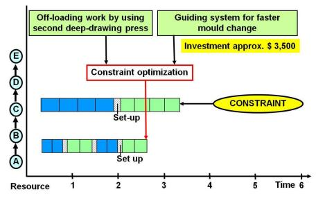
Figure 12: Effect of constraint optimization measures
