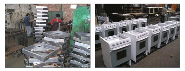
Figure 8: Parts flooding the production floor .... while assembly is waiting for the right parts.
