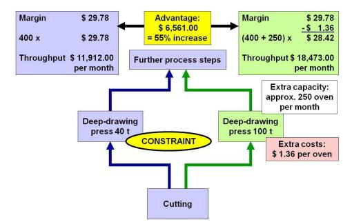
Figure 11: Cost vs. throughput calculations
