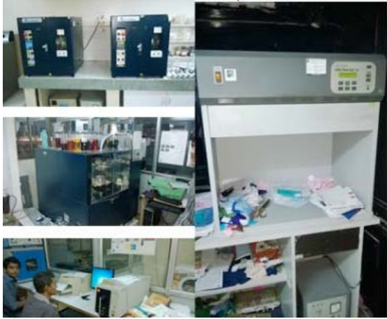
Image no. 27: The auto dispensing system , Spectrophotometer and IR dyer [Source: GIZ-IGEP and GCPC team]
