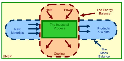
Figure: schematic material and energy balance
