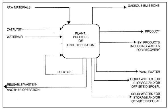
Figure: components of a material balance of a unit operation
