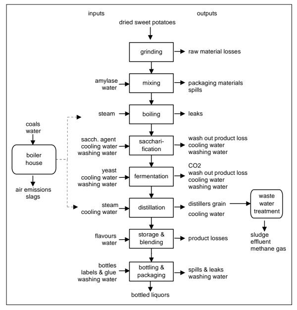
Figure: flowchart derived from an alcohol distillation
