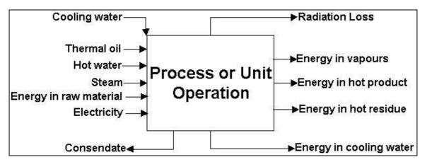
Figure: components for the energy balance
