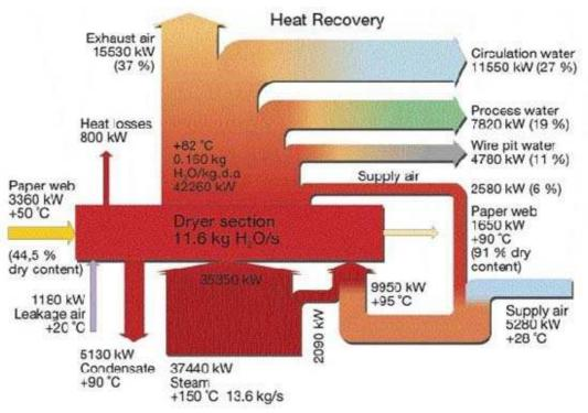
Figure: example Shankey diagram to illustrate the different energy/heat components of a unit operation (dryer)
