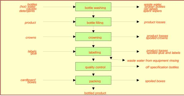
Figure: specific flowchart for the bottling and packaging unit
