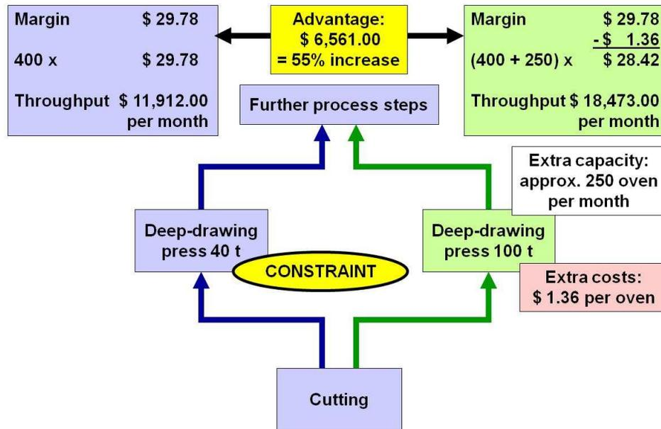
Figure 11: Cost vs. throughput calculations
