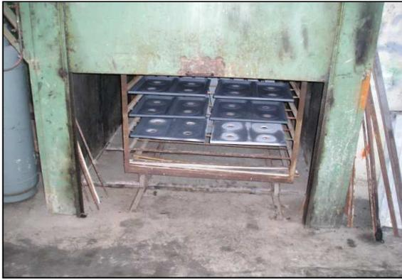
**Figure 6: Batch type electrical furnace**
