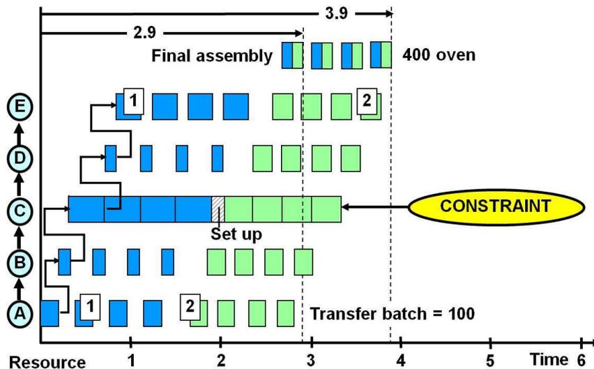
Figure 10: Production with improved flow
