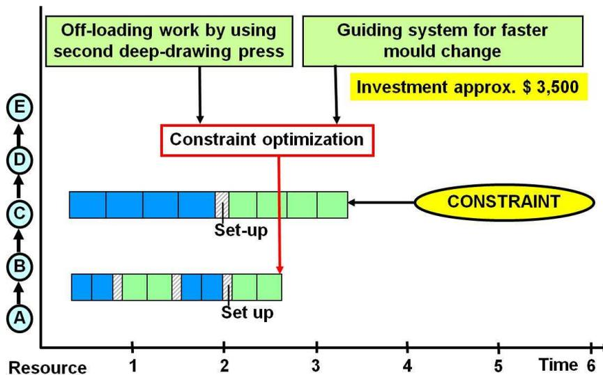
Figure 12: Effect of constraint optimization measures
